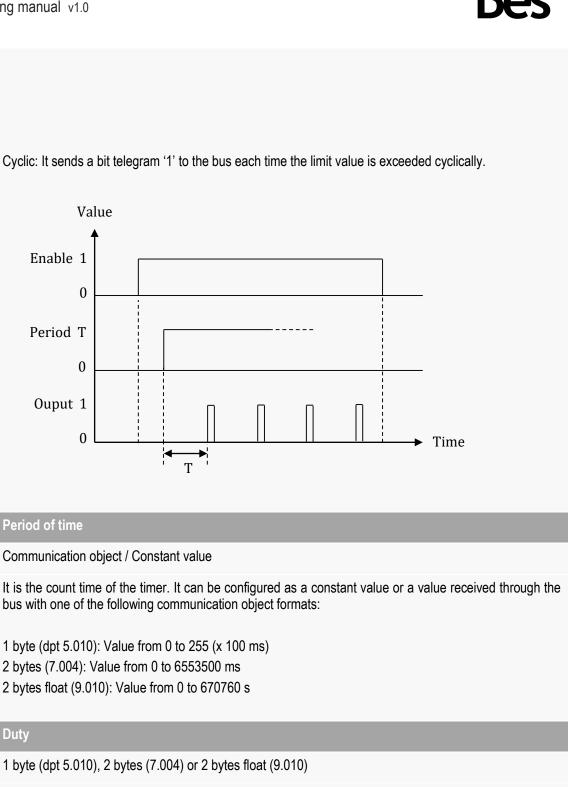
Cyclic: It sends a bit telegram '1' to the bus each time the limit value is exceeded cyclically.
