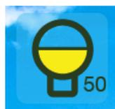
By clicking on the icon, a control dialogue appears and allows to switch on/off the light or setting a new brightness value by sliding the finger (the command is sent when release). It is also indicated graphically as well as numerically the value (in percentage) of the light intensity.
