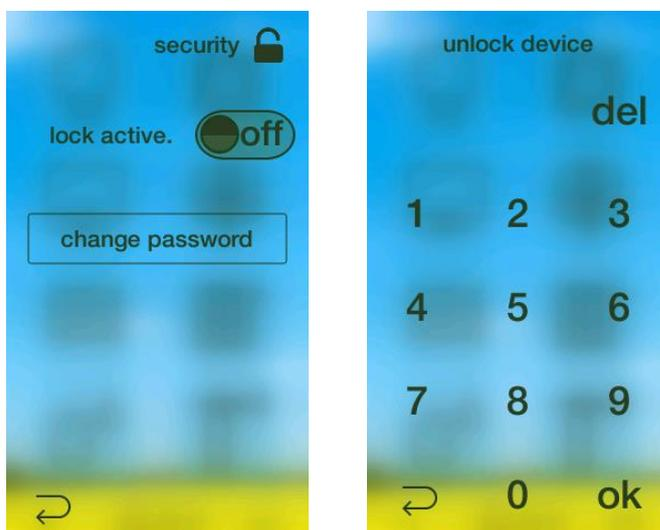
If the lock mode is enabled, the screen will ask for the password every time that changes from standby to active mode. If the lock mode is disabled, the Smart Touch can be activated and therefore used by anyone just by clicking on the screen.
