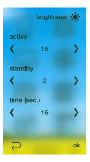
Active [3 - 15]: Is the brightness level when the screen is being used.
