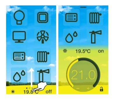
From left to right side it is shown the working mode, the measured temperature and the actual status (on/off) of the internal thermostat.
