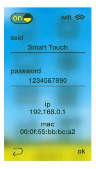
The Wi-Fi network is generated by the Smart Touch with the name (SSID) and password configured in this menu. This network has no internet access, so it is not possible to navigate through the web or control the home automation system from outside the house or installation.
