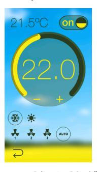
By clicking on this icon, a control dialogue appears and allows to switch on/off the thermostat or setting a new set point temperature by sliding the finger over the circular scroll bar (the command is sent when release). The current measured temperature is also indicated at upper left corner (from 0 to 51 °C).
