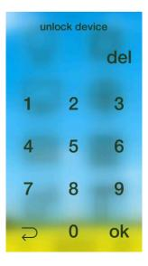
If the lock mode is enabled, the screen will ask for the password every time that changes from standby to active mode. If the lock mode is disabled, the Smart Touch can be activated and therefore used by anyone just by clicking on the screen.
